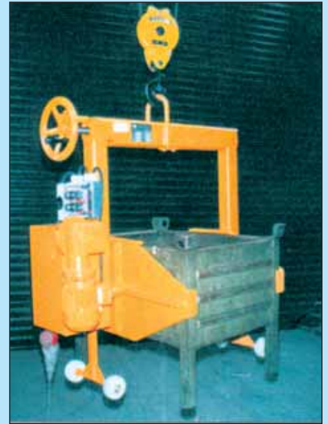
Adjustable beam for storage container with electric drive system
