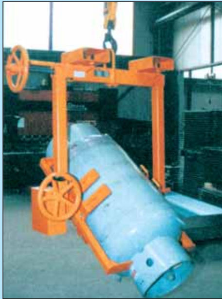
Adjustable beam for boiler with worm gear and hand wheel
