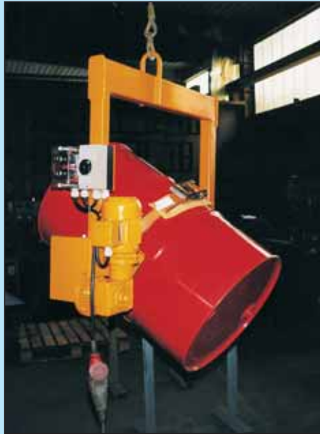
Barrel-tilting beam with electric drive
